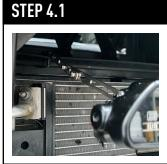
Position the brackets as shown. Drill through the bumper beam (5mm drill) and rivet the brackets to the bumper beam. 4 rivets per bracket.
