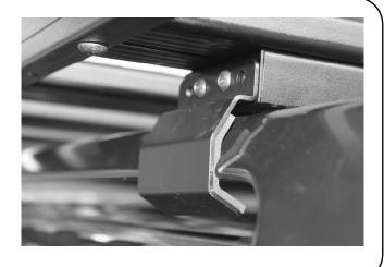
( D ) Insert and firmly fasten two M6 Custom Hex Bolts with two M6 Spring washers and two M6 Stainless Steel Flat Washers. (Items 13, 12 and 11)
