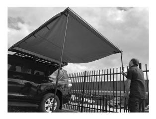
f) Extend horizontal pole so pins on ends of pole, insert into holes in front extrusion & lock in place.
