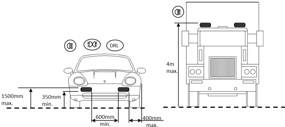
EN : Lamps with integrated DRL and Position light must be positioned according to the above sketch. If an additional pair of position lights is not permitted (e.g. in Switzerland, Austria), the position light should be disconnected. The legal regulations in individual countries must be observed.
